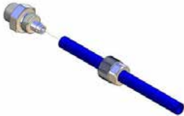
A. Slide a nut over the end of the tube
